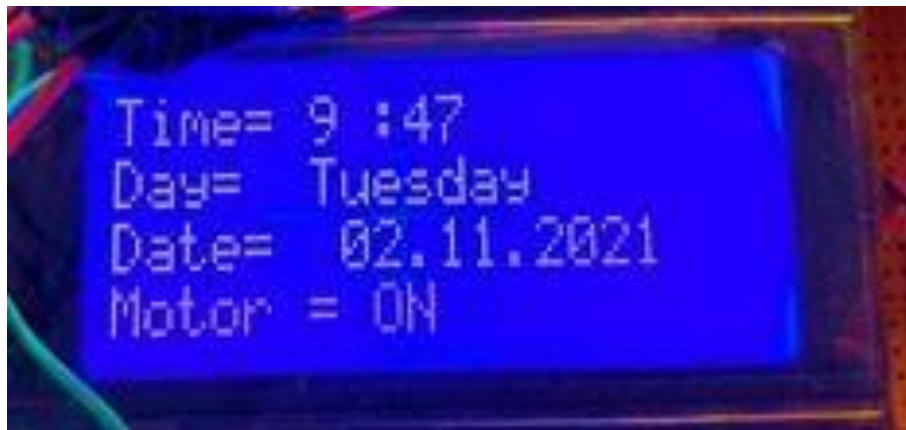
Figure 3: Time and date on the LCD along with the status of motor
