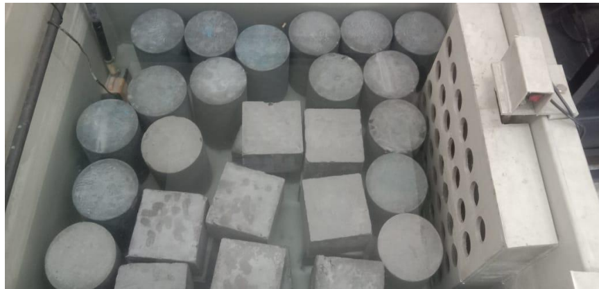
Figure 6. Curing of GFRc cube specimens in a water tank
