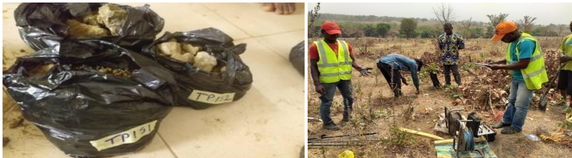
Fig. 4: Collected samples and Posthole hand auger operation of Ihale damsite area
