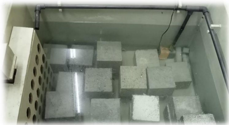
Figure 7. Curing of Concrete Blocks
