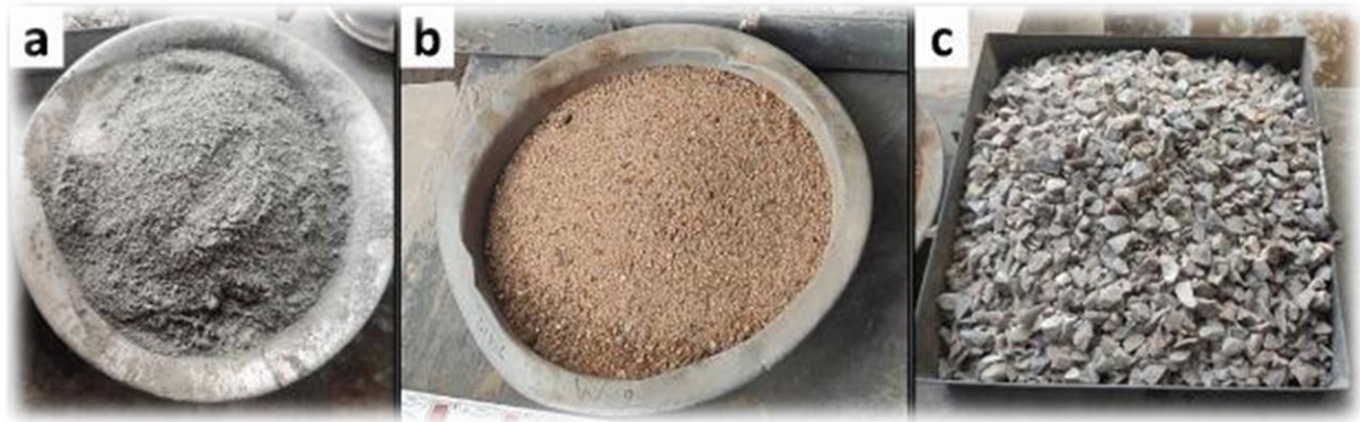
Figure 3. (a) OPC, (b) fine aggregate, (c) coarse aggregate
