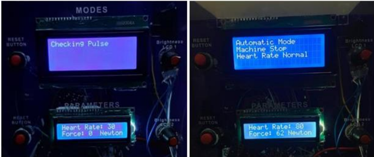
Figure 8. Heart rate Pulse sensor and Force sensor working
