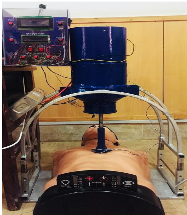
Figure 6. Final Prototype testing on mannequin
