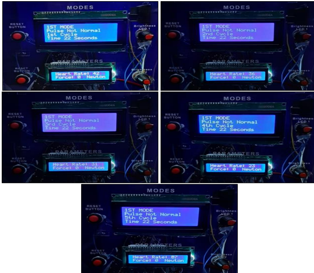
Figure 7. Results of Compressions to Ventilation Mode with multiple Cycles
