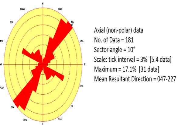
**Figure 12:** Rosette Diagram of the Lineament in the Research Area
