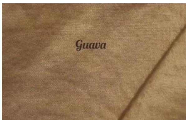
Figure 4: Fabrics after applying guava finish
